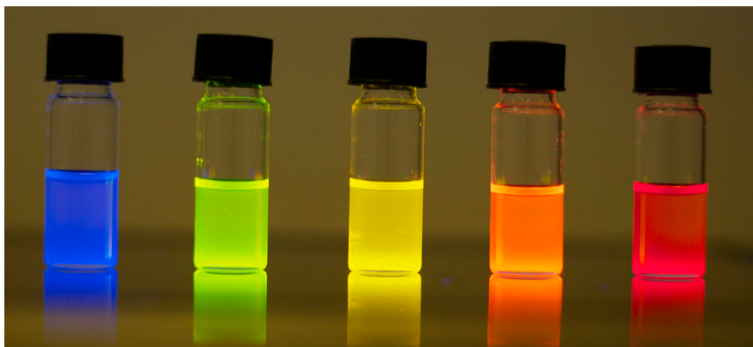
Figure 1. Parisian quantum dots (CdSe/ZnS, courtesy of Benoit Dubertret) shine in bright colors, a beautiful demonstration of the quantum confinement effect in contemporary nanoscience that continues to catch the attention of students and the public alike.
